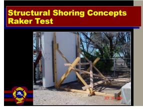
Structural Shoring Concepts Raker Test
